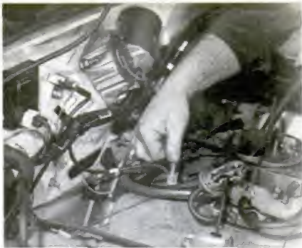
TRACING VACUUM back to manifold: Use your thumb over the nipple when you don't have a vacuum gauge
